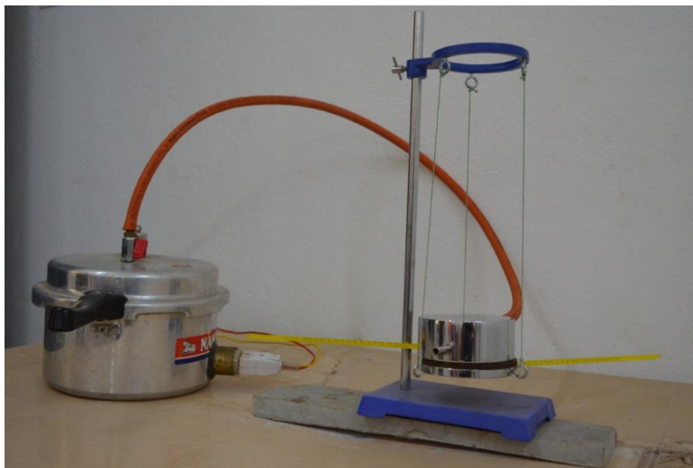
Figure 1. Experimental set up of Lee's disc Apparatus.
