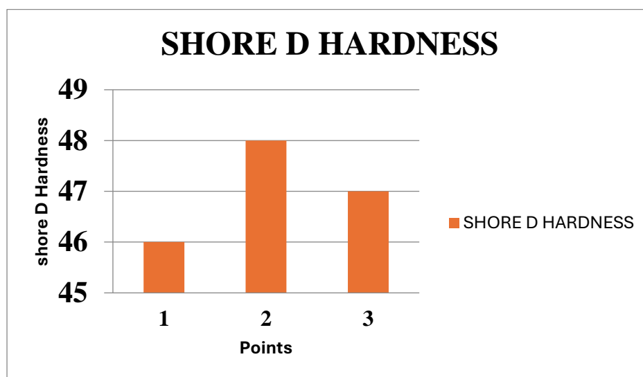
Figure 7. Shore D Hardness for cylindrical mould.
