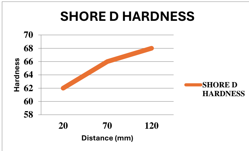
Figure 8. The Shore D-hardness graph for rectangular sample.
