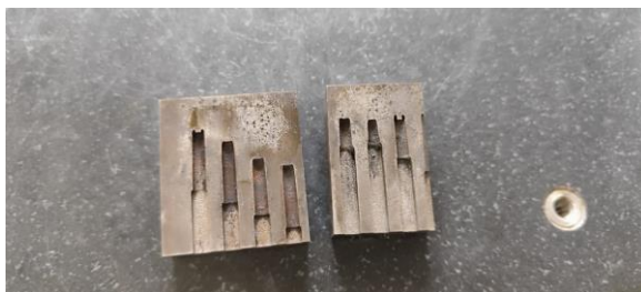
Figure 5. Workpiece samples after wirecut.
